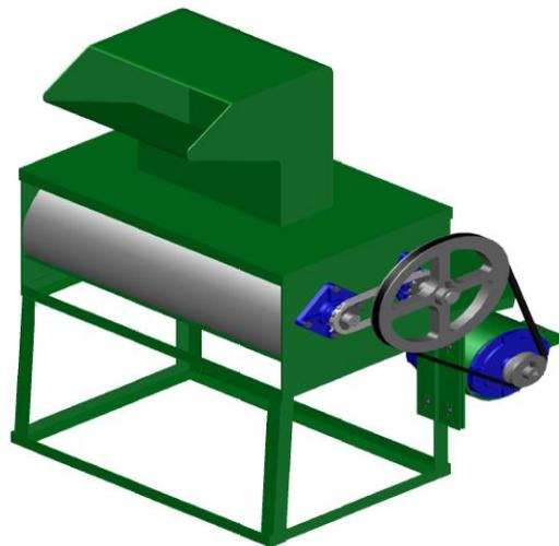
Fig.2: Isometric Modeled View of Groundnut Decortiating Machine
