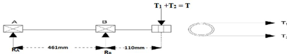
Fig.1 Free Body Diagram of Shaft and Bearing Arrangement
