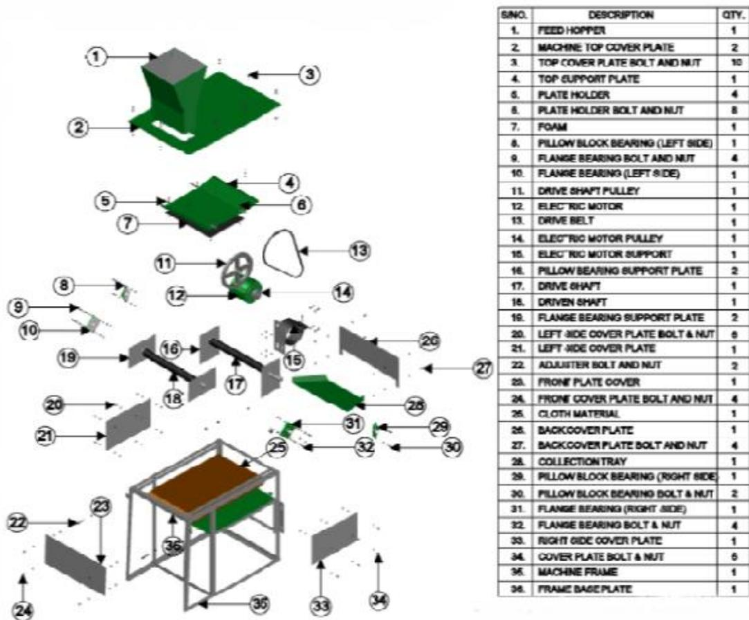
Fig.4: Exploded View of Groundnut Decortiating Machine
