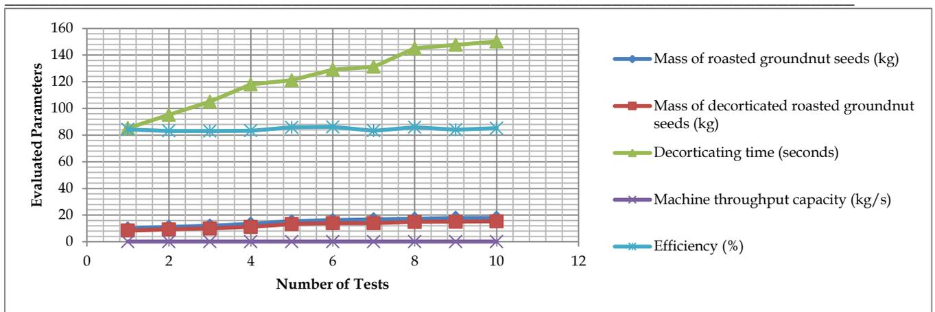
**Fig.5 Graph Performance Test and Evaluation**
