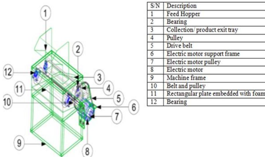
Fig.3: Isometric skeletal View of Groundnut Decortiating Machine
