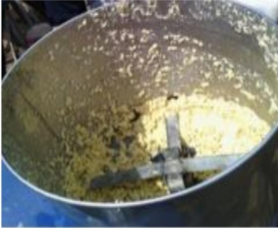
Figure 4: Pulverized Vessel and Product
