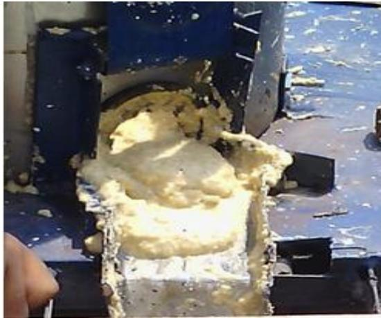
Figure 5: Flow of Plantain Paste through the Pulverizer Outlet
